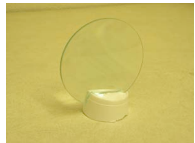
Lens holder made from a Styrofoam cup.
