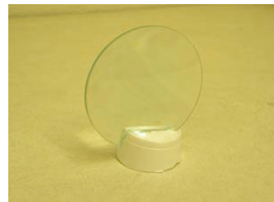
Lens holder made from a Styrofoam cup.
